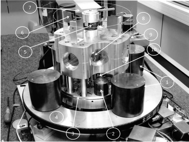
FIG. 1. The BIPM Mk II  $G$  apparatus: 1, Cu-Te 11 kg source masses; 2, Cu-Te 1.2 kg test mass resting on torsion disk (3); 4, aluminum alloy carousel; 5, gimbal from which torsion strip and torsion balance are suspended; 6, eddy-current dampers for gimbal; 7, autocollimator; 8, central mirror tower on torsion balance; 9, position of vacuum can; 10, electrodes for servo control.
