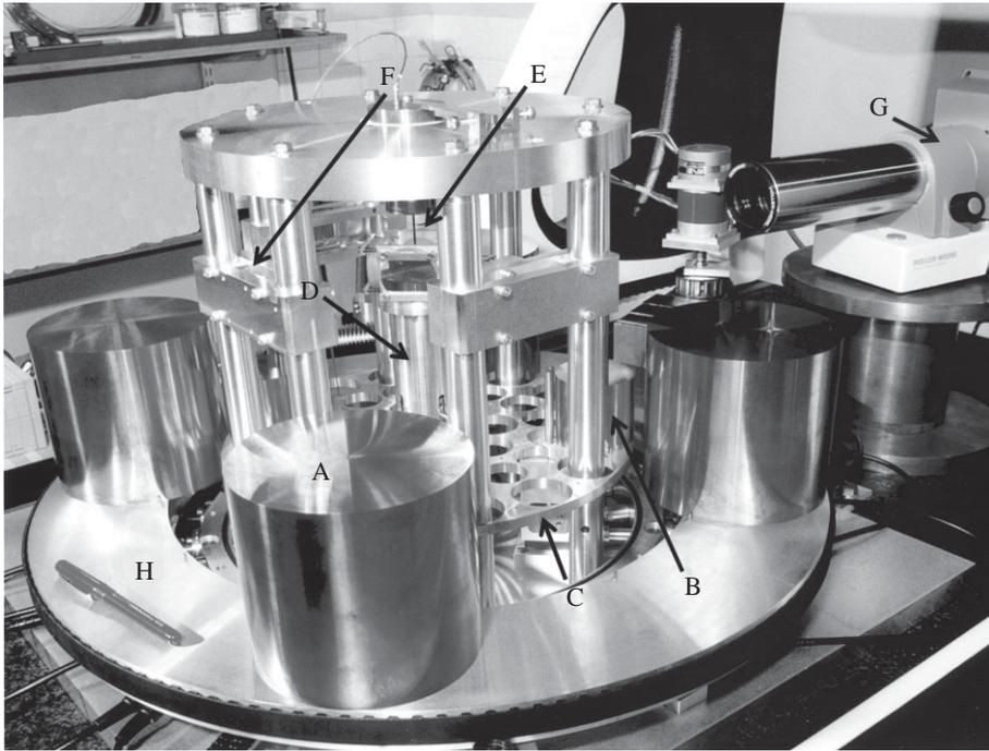
**Figure 1.** The Mk I apparatus: (A) one of the four source masses ( $\approx 11$  kg); (B) one of the four test masses ( $\approx 1.2$  kg); (C) the torsion disc about 30 cm in diameter; (D) the central tower holding mirrors, down the centre of which is suspended the torsion strip, just visible; (F) one of the three mirror supports part of the  $\times 6$  multiplying optics; (G) the autocollimator; and (H) the carousel.
