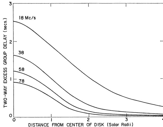
FIG. 3.—Computed excess group delays for the Pottasch density and for rays reflected at the turning points.
