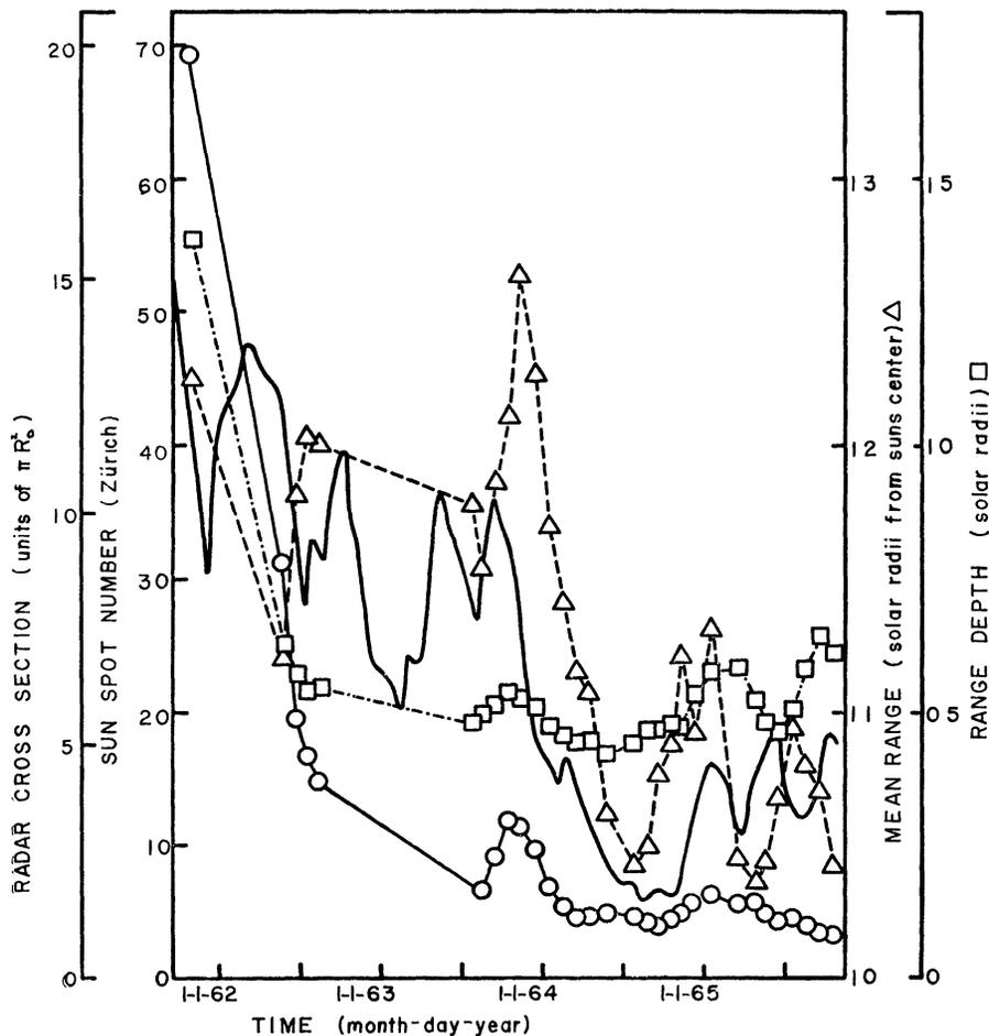
FIG. 5.—The variation of solar radar parameters, as measured at El Campo, and the average sunspot number with time. Each point represents an average of the radar measurements made over a 2- to 3-month period, and the sunspot number plot is a 3-month running average. The cross-section values were adjusted to apply for echo energy received over a wide band, and the mean range values were computed on the basis of an assumed 1.6-sec additional group delay in the corona.
