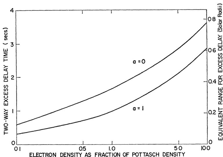
FIG. 4.—Computed excess group delays at 38 Mc/s for a ray directed at the center of the disk ( $a = 0$ ), and for a ray directed at the limb ( $a = 1 R_{\odot}$ ). The electron density throughout the corona is assumed to be multiplied by the factor indicated.
