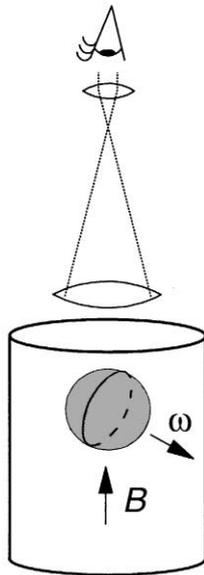
Fig. 1. Experimental setup. Plastic ball is spinning inside a Bitter magnet around the  $\omega$ -axis. A pattern on the surface allows detection of changes in the  $\omega$ -axis’ orientation as earth rotates.
