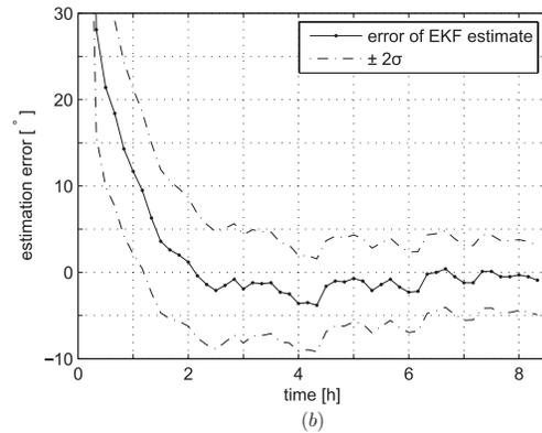
**Figure 7.** Gyrocompassing results obtained in two runs. The initial offset angle was 90° from the east direction in both cases; the first estimates have been cropped out.
