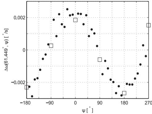
**Figure 6.** Differenced angular rates (3) from a 450° rotation spaced by 10°. Observations made at the principal compass points are denoted by squares.
